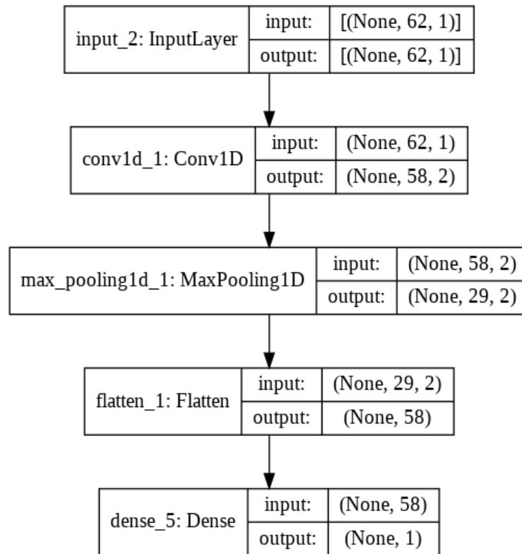
**Fig 2: Neural Network model graph obtained for CNN**
